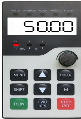
Figure 4-6 Frequency converter power-on display
