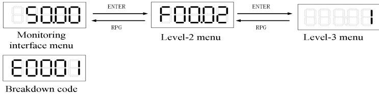
Figure 4-4 Operation hierarchy diagram of level of verify menu
