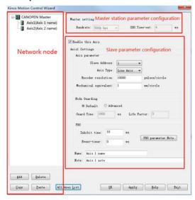
The window is divided into three parts: a tree list of network nodes, parameters of the master station, and parameters of the axis (slave).
