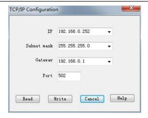
In a local area network, PLCs and PCs located in the same network segment (that is, the first three numbers of the IP address must be the same and the last one different) can communicate with each other.
