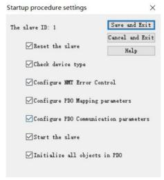
[Reset Node]: Whether the master station sends the "Reset Node" command before sending the configuration command to the slave station.
